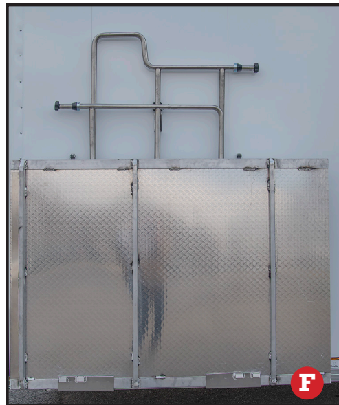
Center ADA ramp on Base with top side facing toward trailer. See image F .
